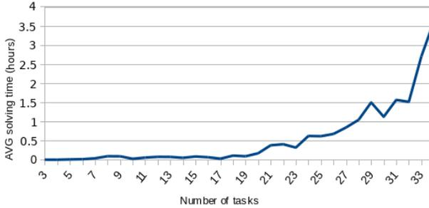
Fig. 3. Scalability of ILP formulation (synthetic task graphs / STG)
